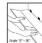
Assemble the second row on the subfloor, tilt and push to attach to the first row, then click into place.
