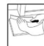
Trim door frames by placing a plank upside down next to the frame and cutting to the necessary height.
