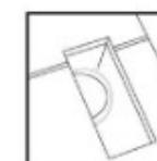
For heating vents, cut the plank to length, measure and mark areas to cut out, then cut allowing for expansion.
